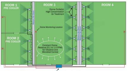
Ensure™ Ozone System Location (built-in monitor/controller)
